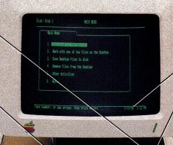
Real-time clock displays time and date on AppleWorks™ screens and files, and is PRO-DOS compatible for use with other PRO-DOS software.
